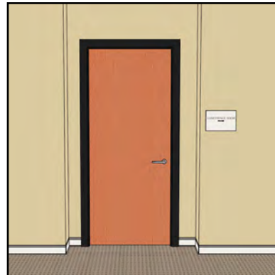
Recessed door with sign on adjacent wall
