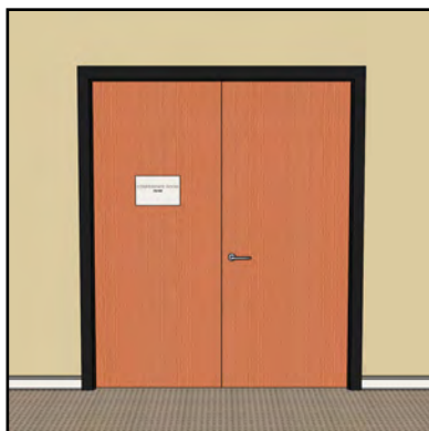
Sign on inactive leaf at double-door entry
